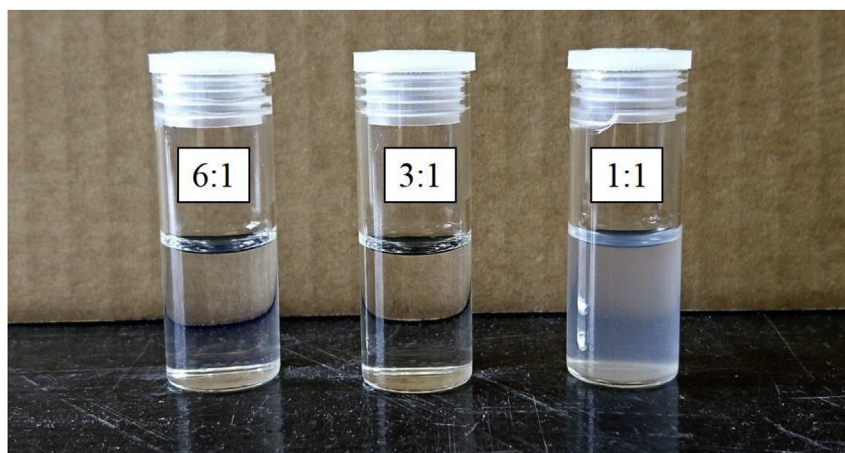
Fig. 1. Visual Image of chitosan nanoparticles at pH 4.6 in 6:1, 3:1 and 1:1 CS:TPP mass ratios (from left to right) where 1:1 is the most turbid while 3:1 is least turbid.
